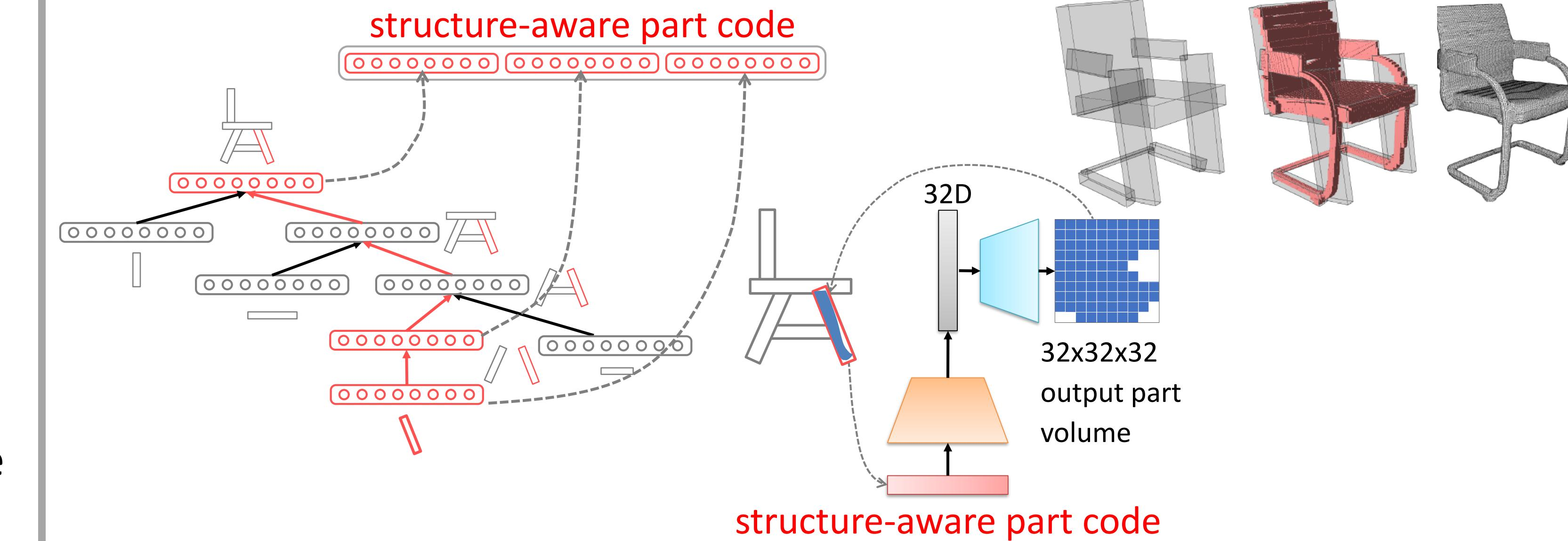
Learn a neural network to map the structure-aware part code of a part into a 3D volumetric representation of its part geometry.
