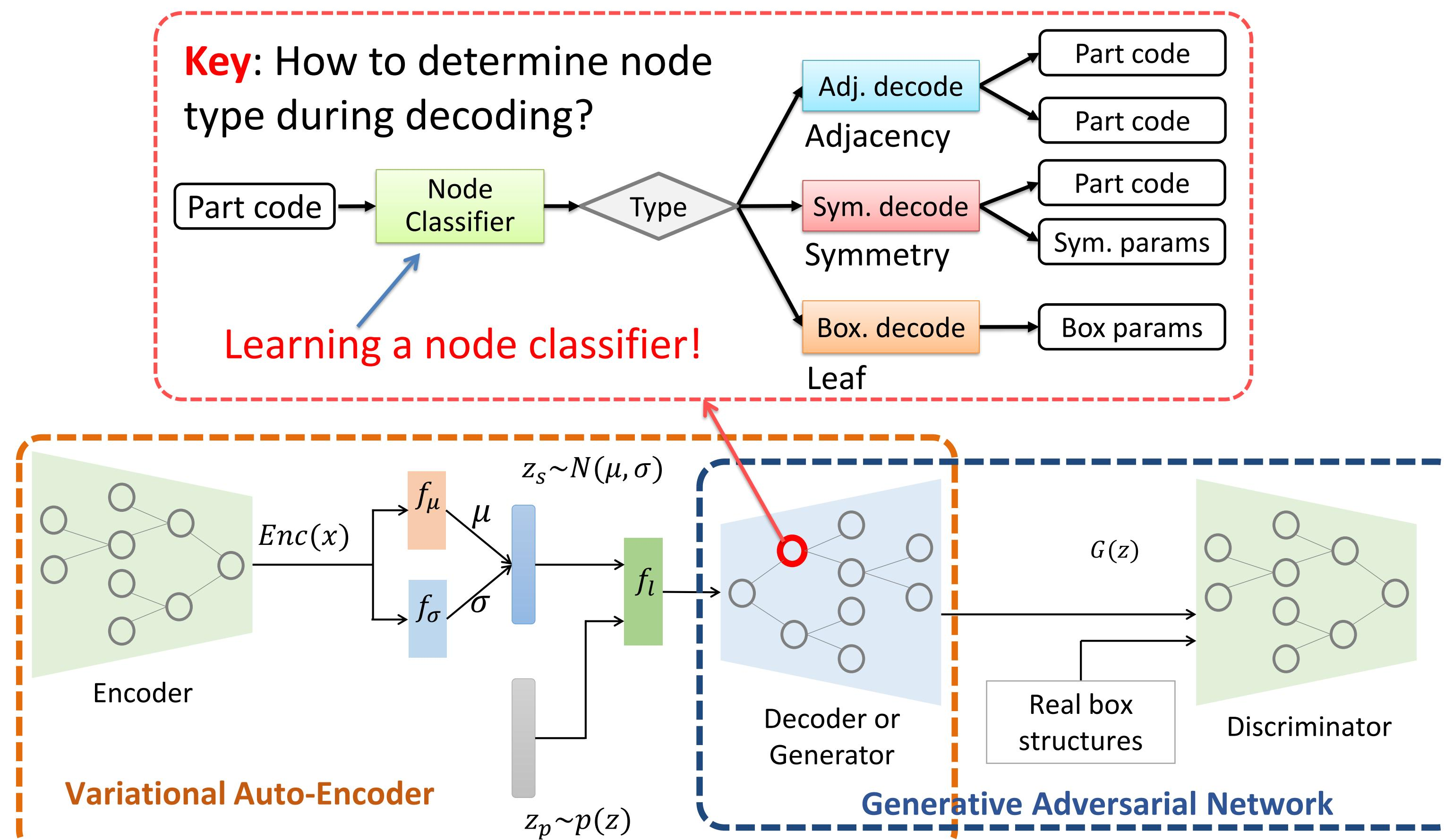
Learn a *probabilistic* generative model to generate novel 3D shape structures – A hierarchy of cuboids encompassing parts and their relationships.
