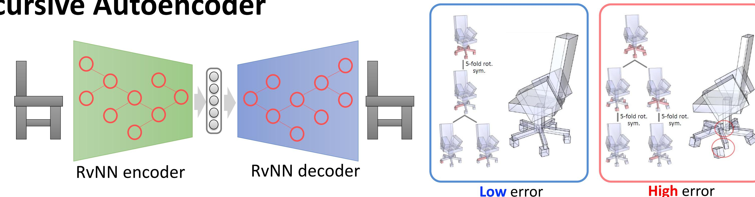
Learn a *deterministic* generative model to find the right hierarchy for structure encoding – The hierarchy that gives the lowest self-reconstruction error.
