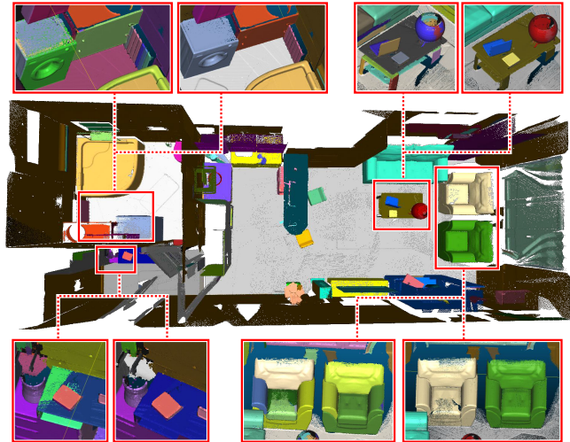
Fig. 6. Four regions in the scanned scene (middle row) are zoomed and their segmentation results of pre-segmentation (left) and post-segmentation (right) are shown side by side for comparisons.
