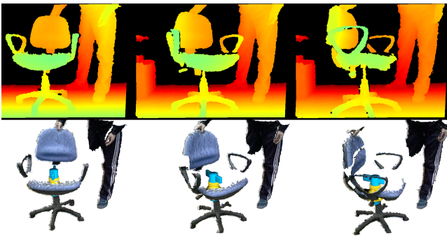
Figure 8: Mobility reconstruction of a manually operated rotating chair. Top row are three frames from the scanned motion. Bottom row shows the reconstructed hinge joint fitted to scans.
