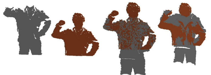
Fig. 6. Alignment of partial scans of human body. From left to right: initial configuration, alignment computed by our method, and by ICP.
