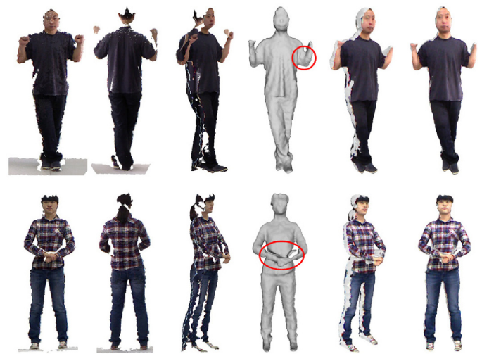
Fig. 12. Two failure cases where the bodies are occluded (red circle) and the reconstructed geometry is incorrect. (For interpretation of the references to color in this figure legend, the reader is referred to the web version of the article.)
