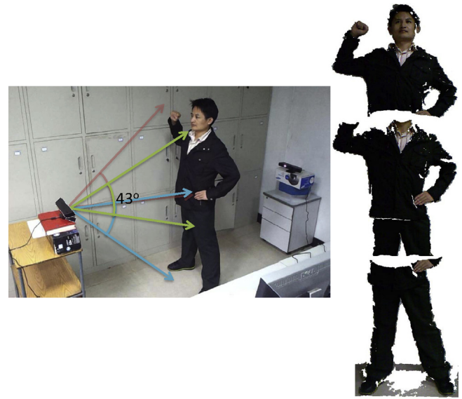
Fig. 2. A snapshot of our system (left) and three partial scans covering the upper, middle and lower part of the human body captured by the front Kinect.
