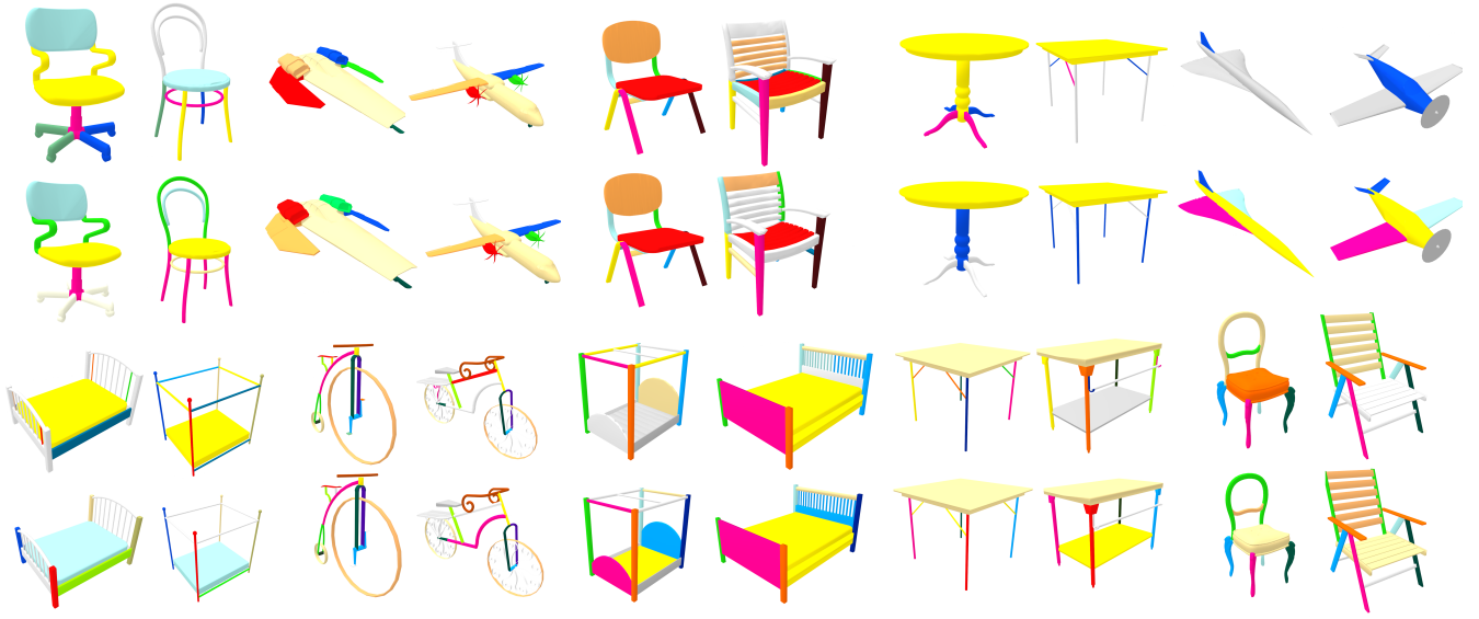
Fig. 11. A gallery of part correspondences computed by our algorithm (bottom pair of each two shape pairs compared) with comparisons to GeoTopo [Alhashim et al. 2015]. Matched parts share the same color; unmatched parts are in gray.
