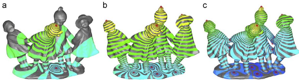
Fig. 1. Iso-contour plots of harmonic fields over the high-genus children model (304K vertices), where red dots mark the chosen sites. Iso-contour strips are colored via linear interpolation between blue (value 0) and yellow (value 1). Updating time is less than one second, allowing for exploration of varying design choices in real time.
