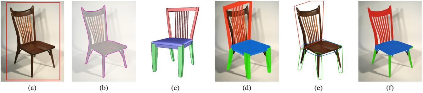
**Figure 5:** Steps of model-driven object segmentation. Given an input photograph, the user draws a box (a) to seed a graph cut algorithm and produce a rough object silhouette (b). A 3D model (c) is retrieved based on the silhouette, then overlaid onto the photo (d). Convex hulls of the model parts (e) provide seeds to a multi-kernel graph cut to produce the final segmentation (f); color labels reflect object parts.
