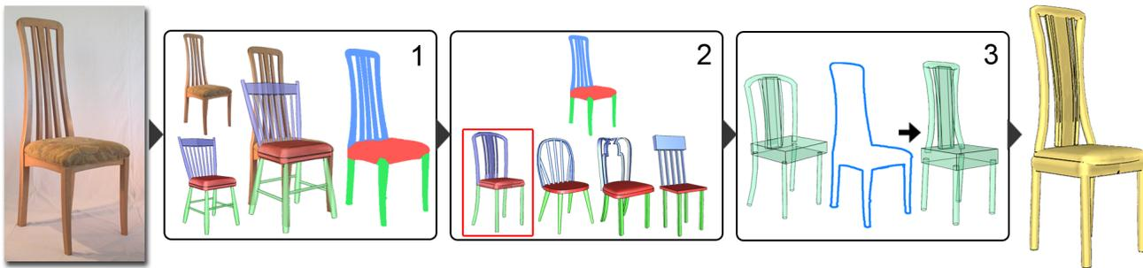
**Figure 4:** Overview of photo-inspired 3D modeling. Given a single input photograph, a model-driven approach is applied to obtain a labeled segmentation of the photographed object (step 1). The candidate to be deformed can be randomly chosen or retrieved from the candidate set (step 2). The chosen candidate is deformed to achieve a fit in the silhouettes while preserving its structure (step 3).
