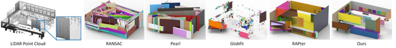
Fig. 10. Comparison to the other methods on raw LiDAR data with *density anisotropy*. All methods reconstruct dominant planar structures, except Globfit. The relatively smaller structures, like windows, are successfully obtained from our method, which, however, are missing from the others.
