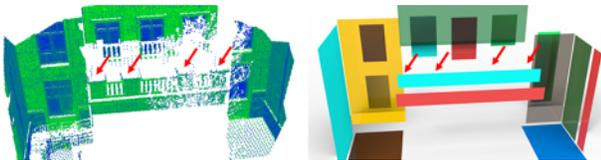
Fig. 16. The points on the top faces of the columns are significantly missing. Consequently, our local classification fails to detect the top patches.
