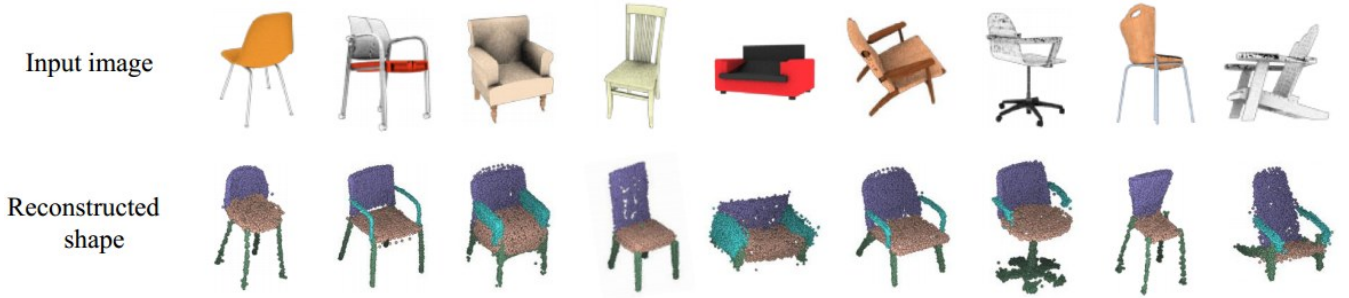
Figure 2: Reconstruction results of the proposed pipeline with known camera pose. RGB images are the input, the results are colored according to the part label: seat (olive), back (purple), armrests (blue) and legs (green).
